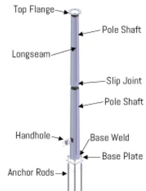
An unmitigated failure, if one was to occur at this joint, will in almost all cases be catastrophic resulting in the collapse of the pole.
