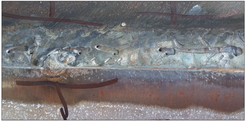
Tower modification weld with example of elongated porosity.
