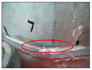
Toe Crack Visible via MT Powder after Grinding
