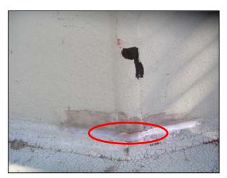
Minor Toe Crack Visible via MT Powder after Light Grinding
