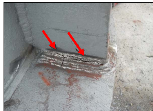
Stiffener Longitudinal & Transverse Cracks (in Black)
