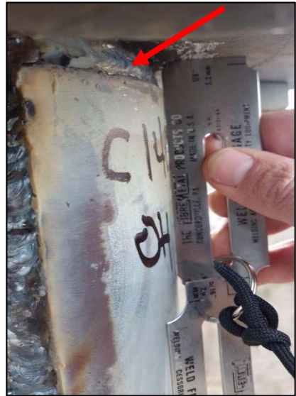
Tower Leg Split Pipe Modification Incomplete Joint Penetration to Leg Flange
