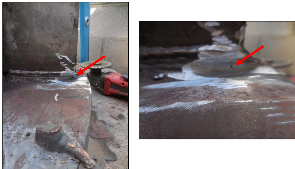
Monopole Base Plate Stiffener Weld CJP Connection Slag Inclusion
