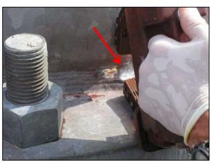
MT Exam Showing Indication (Crack) at Upper Toe
