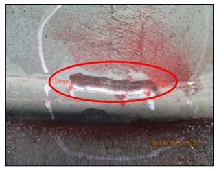
Toe Crack Still Visible via MT Exam after Grinding
