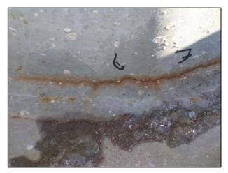
Toe Cracks at Upper Toe of Weld in Pole Shaft at Polygonal Bend Line (Visible Rust)
