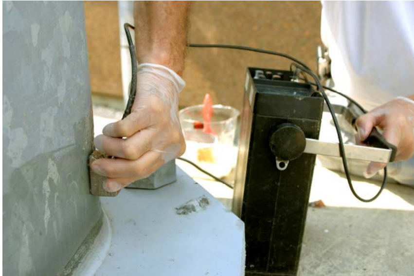
Ultrasonic Test (UT) of Pole Base Plate Weld
